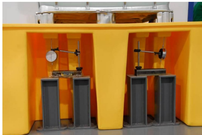
Measure the deflection of the pallet
